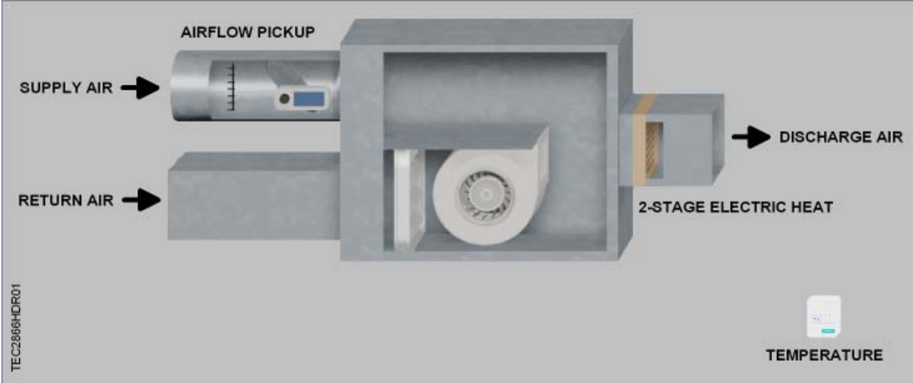
Application 2866 with Parallel Fan and 2-Stage Electric Heat Hardware Diagram
